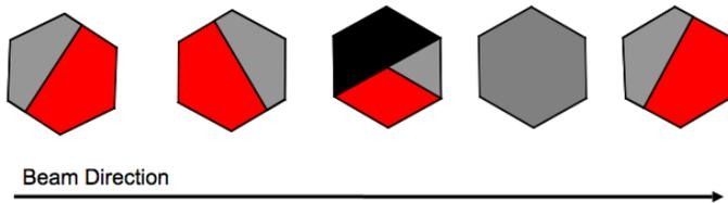
Fig. 3. Geometry of the nuclear targets in MINER $\nu$ A. The targets are stacked in the detector in the order shown, from left to right. Four scintillator modules are placed between each target. Deep gray (red): Fe, grey: Pb, black: C.
