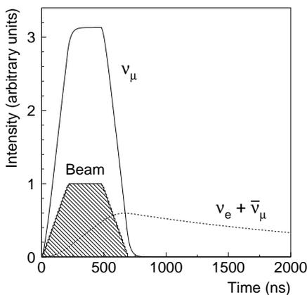
Fig. 2. Time structure of the different neutrino species produced at the SNS.
