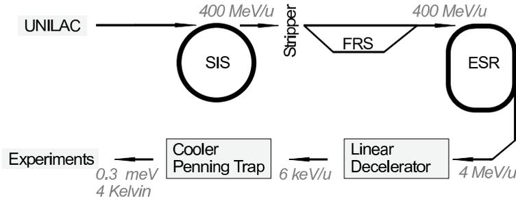
Fig. 1. The HITRAP facility at the GSI accelerator complex.
