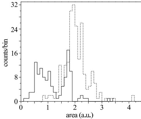
Fig. 2. Signal on the diamond detector binned by peak area, which is proportional to the impinging ion’s energy, with the radio frequency of the IH structure switched on (solid line) and off (dashed line).
