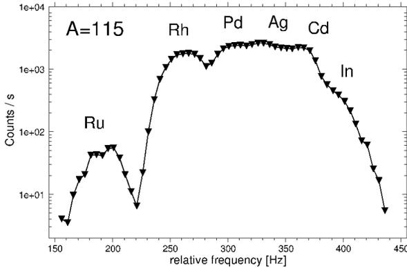
Fig. 1. Ion counts registered with the MCP detector during a wide range frequency scan of the quadrupole electric field in the trap. The well resolved atomic ions from the IGISOL isobaric beam are marked with an element symbol.
