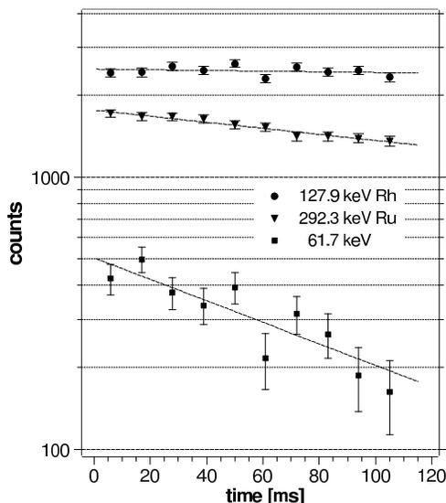
Fig. 4. Decay of 292.3 keV and 127.9 keV gamma lines which are the most intensive transitions fed in  $\beta$  decay of  $^{115}\text{Ru}$  and  $^{115}\text{Rh}$ , respectively. At the bottom the decay of 61.7 keV which may be an isomeric transition. The half-lives measured in this work are 270(38) ms for 292.3 keV and 76(14) ms for 61.7 keV.
