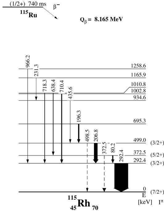
Fig. 3. A partial  $^{115}\text{Ru}$  beta decay scheme as obtained in the present work. The 292.3 keV transition was found with the IGISOL [8], later the 80.2, 196.3 and 206.8 keV gammas were found in a trap assisted study [4].
