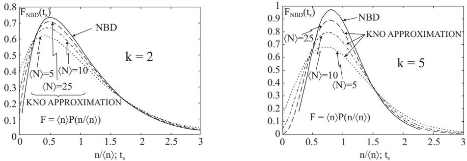
Fig. 2. KNO approximation for the Negative Binomial Distribution. Full line: the function  $F[t_s(n)]$  evaluated from (13); other lines:  $F[t_s(n)]$  obtained from KNO approximation (10) for various  $\bar{n}$  (as indicated in the figure). One sees an apparent violation of the KNO scaling even at  $\bar{n} = 25$ .
