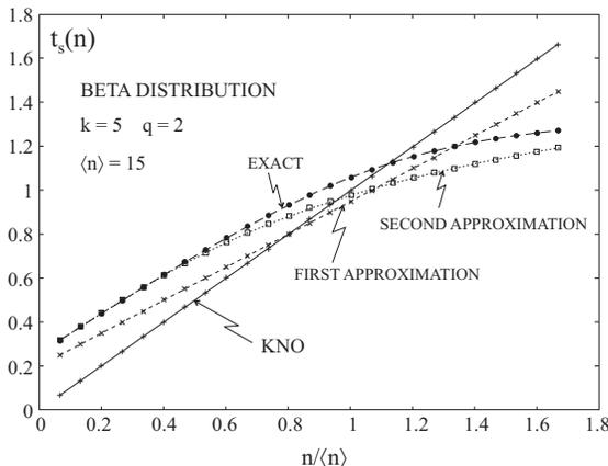
Fig. 4.  $\beta$  distribution (30).  $t_s(n)$  is plotted *versus*  $\bar{t} = n/\bar{n}$ . One sees that the first order approximation (being linear) cannot reproduce the exact result. The second order approximation gives good agreement at  $n < \bar{n}$ . The discrepancy persists, however, at larger  $n$ .
