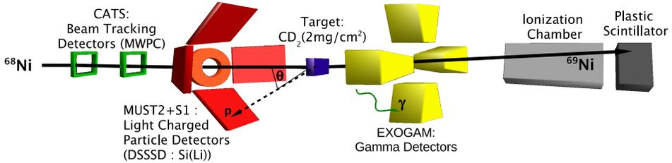
Fig. 1. Schematic drawing of the experimental setup showing respectively from left to right, two beam trackers (CATS), a set of light charged particles detectors (MUST2 and an annular DSSSD), a  $\text{CD}_2$  target, four  $\gamma$  rays detectors (EXOGAM clovers), an ionisation chamber and a plastic scintillator. The proton emission angle is calculated event by event, between the ion trajectory and the proton trajectory as shown in the drawing.
