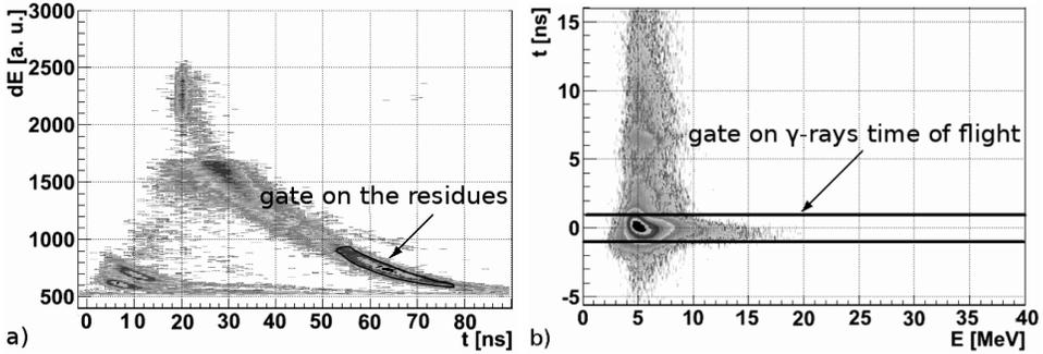
Fig. 1. (a) Energy loss ( $dE$ ) in the first layer of the phoswich detector [16] versus time of flight. The marked region corresponds to the detection of residues. This gate is used to produce the clean high-energy  $\gamma$ -spectra. (b) The time of flight versus energy measured with the HECTOR detector. The gate indicated selects  $\gamma$ -rays without influence of neutrons energy deposits.
