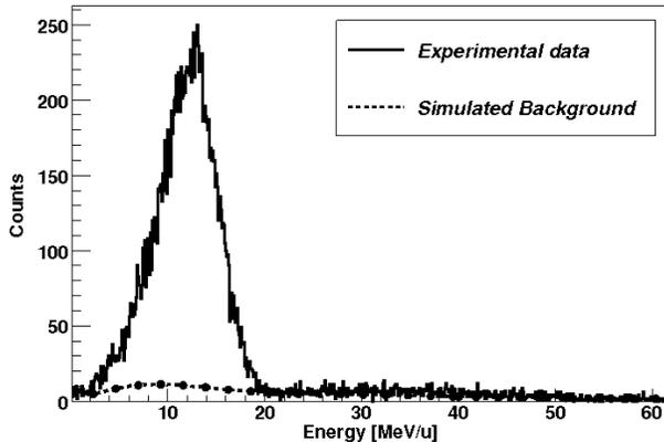
Fig. 4. Energy distribution of  $^{64}\text{Ni}$  ions after slowing down in Al degrader. A final energy of 13 MeV/u was obtained with a width of 8 MeV/u. The dashed curve represents the simulated background.
