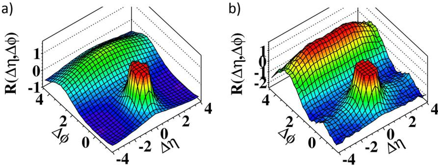
Fig. 1. Two particle correlation function for 7 TeV  $pp$  for intermediate  $p_T$  range, minimum bias events (left) and high multiplicity events (right). The sharp near-side peak from jet correlations is cut-off in order to better illustrate the structure outside that region [1].
