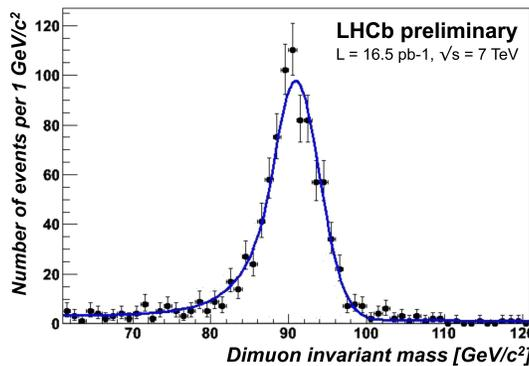
Fig. 2. Invariant mass of the dimuon system. The data points are fitted to a Gaussian on a polynomial background.
