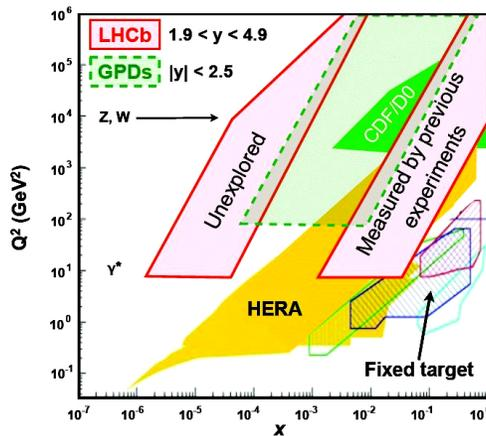
Fig. 1. The kinematic region  $x - Q^2$  probed by the LHCb experiment with electroweak boson production together with the region probed by Tevatron, HERA and fixed target experiments.
