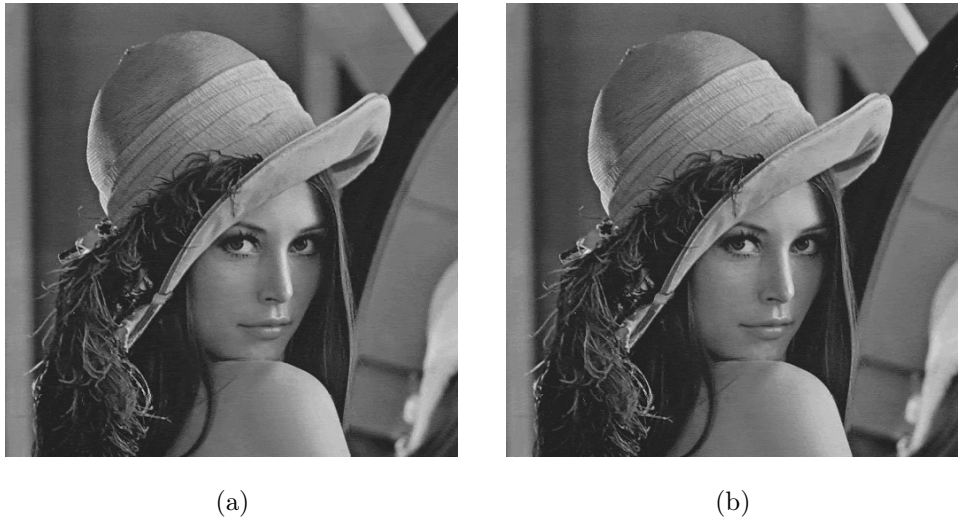
Fig. 2. The decompressed image of Lena for (a) previous method [17] — compression ratio:3.2; PSNR:34.5 dB, (b) new method — compression ratio:3.3; PSNR: 34.6 dB (quant accuracy:5, noise ratio:2).
