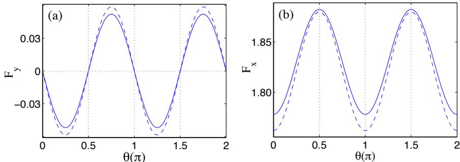
Fig. 3. The dependences of lift force  $F_y$  (a) and drag force  $F_x$  (b) on  $\theta$  for the fixed distance  $r = 12$ , which corresponds to the dashed line circle in Fig. 2. The solid lines are calculated results and the dashed lines are fitted results using Eq. (8).
