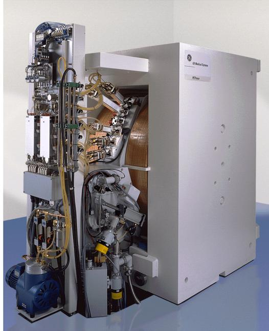
Fig. 1. The GE Healthcare PETtrace cyclotron, accelerating protons with energy of 16.5 MeV and deuterons with energy of 8.4 MeV with proton current up to  $100 \mu\text{A}$ . This type of cyclotron will be operational at the beginning of 2012 in the Radiofarmaceuticals Production and Research Centre of the Heavy Ion Laboratory, University of Warsaw (courtesy of GE).
