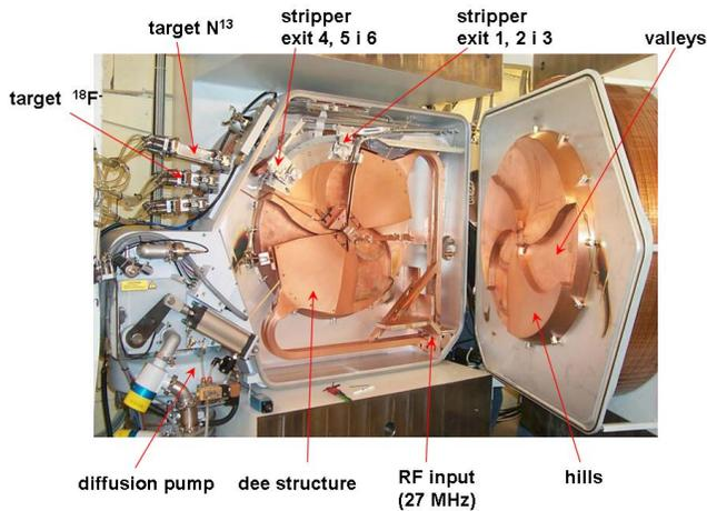
Fig. 2. Interior of the PETtrace cyclotron (courtesy of GE).
