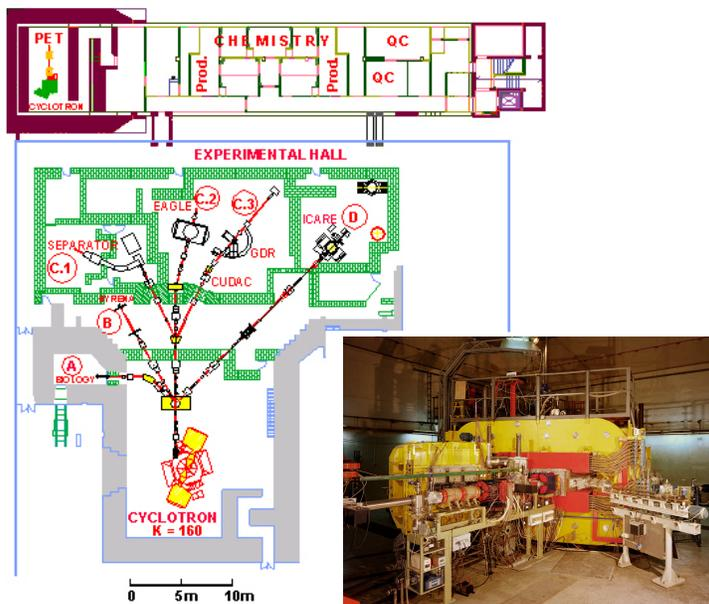
Fig. 4. Layout of the ground floor of the HIL building. Lower part of the layout shows the heavy ion cyclotron, the beam lines and the nuclear physics experimental stations. Upper part shows the Radiopharmaceuticals Production and Research Centre, placed underground ( $-7\text{m}$ ), see also [www.sl.cj.uw.edu.pl/pet](http://www.sl.cj.uw.edu.pl/pet).
