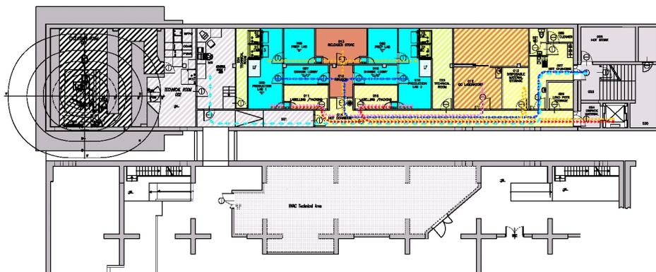
Fig. 5. Layout of the RPRC. Proton/deuteron cyclotron and its control room is placed on the left part of the figure. Two independent production rooms are placed in the middle of the figure (The first one for the routine production of FDG and the second one for other radiopharmaceuticals). The Quality Control room is placed in the right part of the figure.
