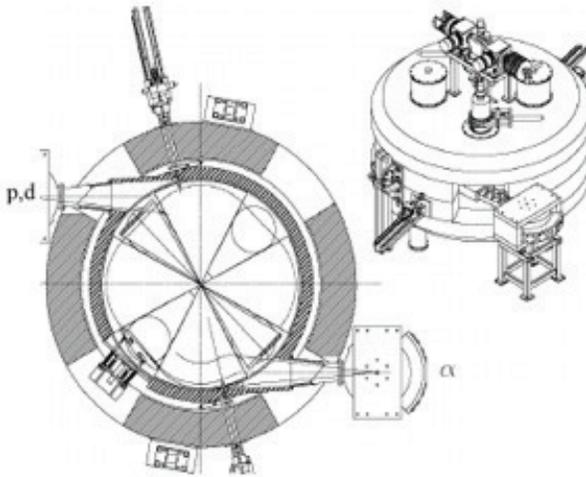
Fig. 3. Schematic and cross-sectional view of the IBA CYCLONE XP 30. Two ion sources (multicusp and ECR) are shown on the top of the cyclotron (courtesy of IBA).
