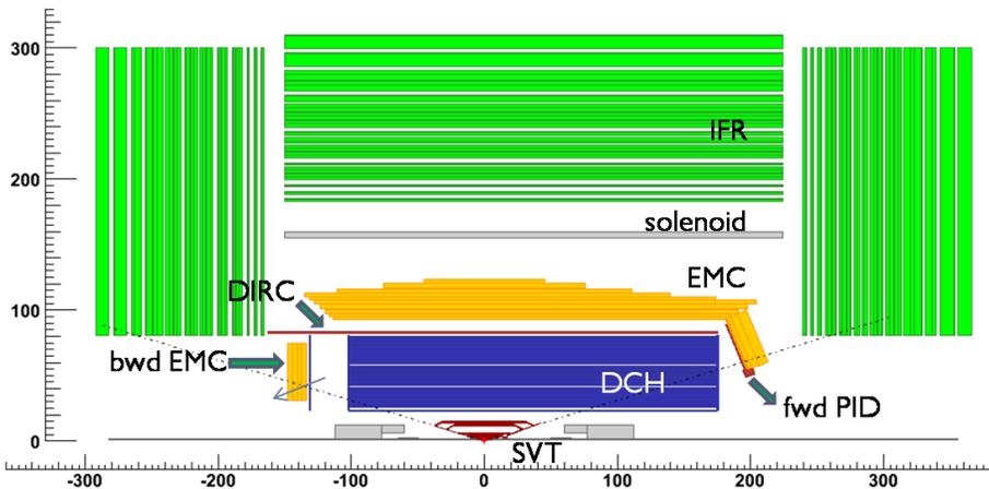
Fig. 2. Concept for the SuperB detector.
