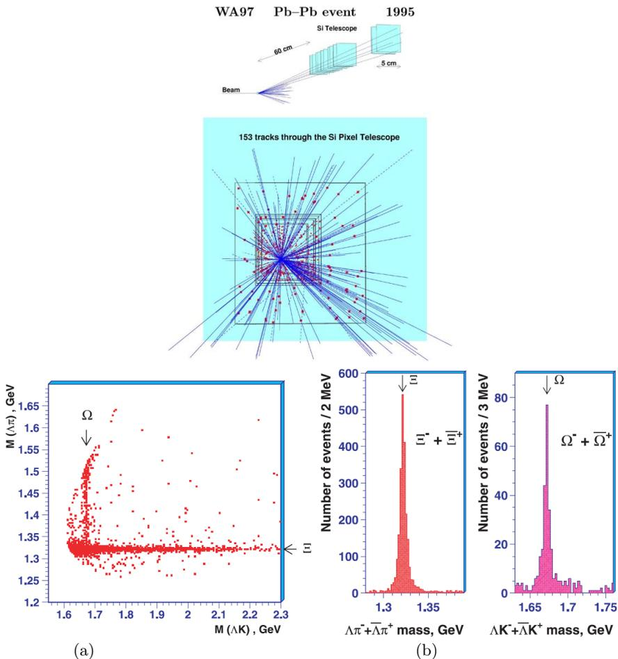
Fig. 4. WA97: (a) A reconstructed Pb–Pb event, recorded in the absence of magnetic field. It contains 153 tracks, *i.e.* an occupancy of about 0.2% of the channels. (b) Identification of  $\Xi$  and  $\Omega$  hyperons.
