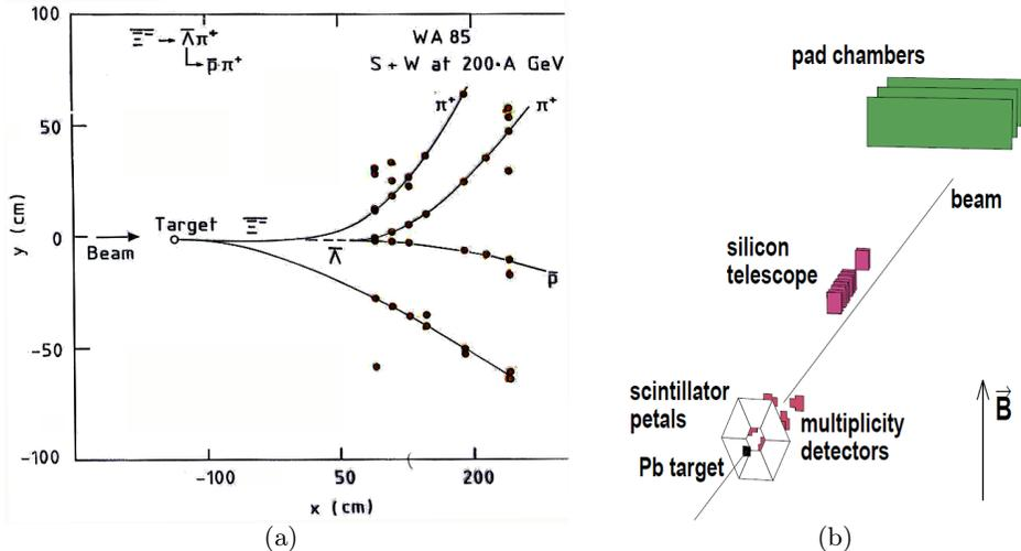
Fig. 2. (a) WA85: fully reconstructed decay of a  $\Xi^-$  produced in a central S–W collision at 200 A GeV. (b) WA97 layout: multiplicity detectors to provide a centrality trigger, compact silicon telescope, lever-arm pixel planes followed by wire chambers with pad cathode readout.
