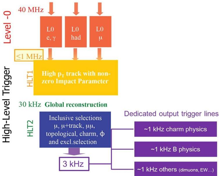
Fig. 3. Schematic drawing of the LHCb trigger system.
