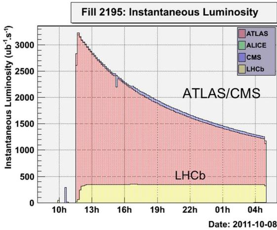
Fig. 4. Example of luminosity leveling throughout a physics fill. The LHCb delivered luminosity is kept constant as opposed to the delivered luminosity in ATLAS and CMS.
