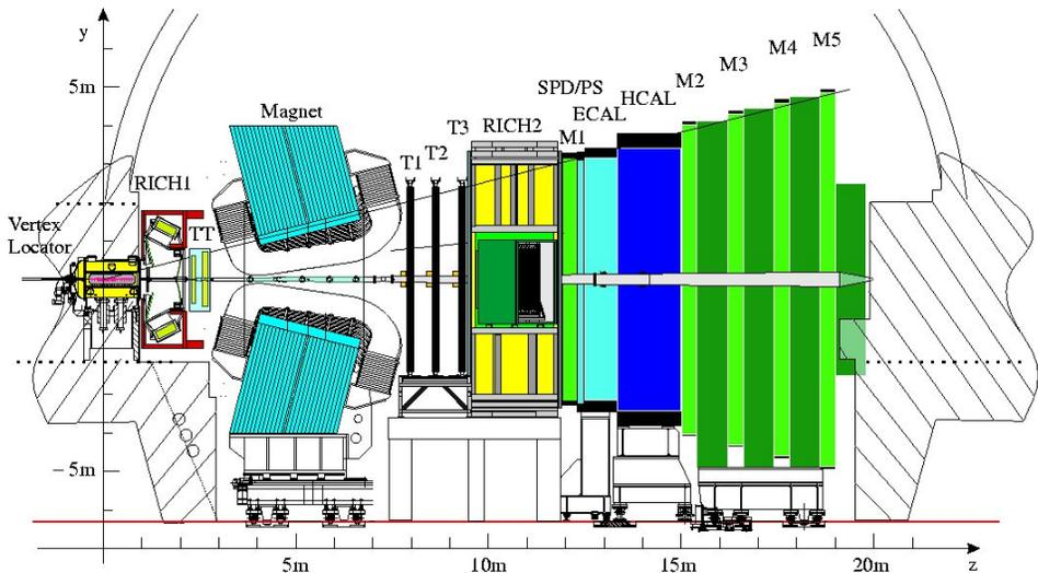
Fig. 1. The layout of the LHCb detector.
