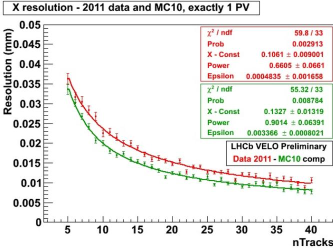
Fig. 2. VELO resolution of primary vertex location as a function of the number of tracks.
