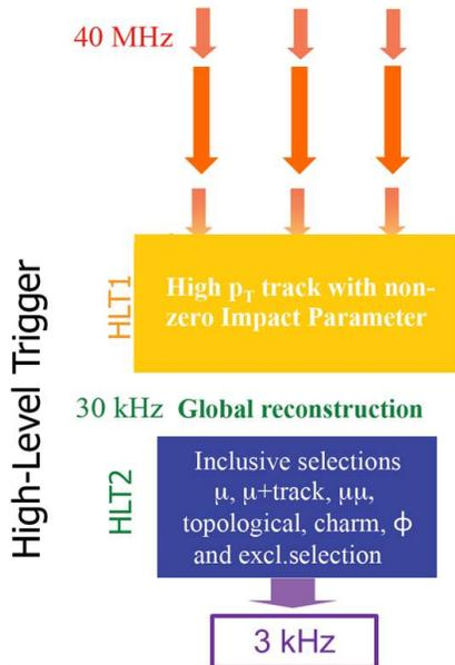
Fig. 10. Schematic drawing of the upgraded trigger architecture as compared to figure 3. The first-level trigger is suppressed and the full set of events is available to the farm to be analyzed and processed. In reality, a *Low Level Trigger* will still be present between the Front-End electronics and the Back-End electronics in order to allow for a staged upgraded readout architecture and also for rate regulation of the system in case needed.
