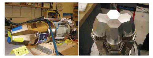
Fig. 6. GRETINA quad module showing the 4 canisters inside the cryostat.
