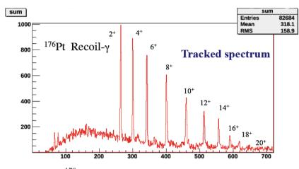
Fig. 7. Spectrum of <sup>176</sup>Pt in coincidence with recoils at the focal plane of the BGS.
