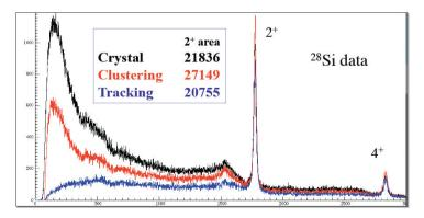
Fig. 8. Reconstructed spectrum for  $^{28}$ Si from the commissioning run at NSCL. The improved quality after tracking is observed.
