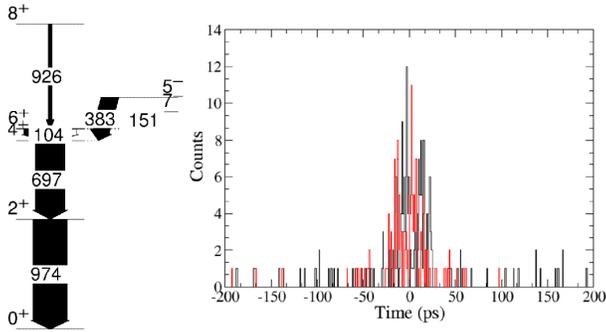
Fig. 1. Left: A partial level scheme for  $^{132}\text{Te}$  up to  $I^\pi = 8^+$ . Right: The forward and backward time spectra for the 383 and 697 keV transitions which show a Gaussian distribution, indicating  $T_{1/2} \leq 40$  ps for the  $4^+$  level in  $^{132}\text{Te}$ .
