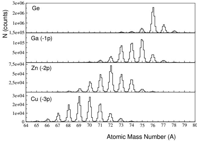
Fig. 1. Isotope yield for Ge, Ga, Zn and Cu. The statistics shown consider all distances measured in the experiment.
