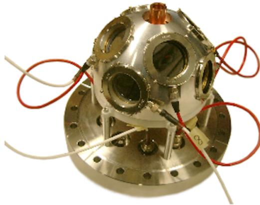
Fig. 3. Picture of the scattering chamber. The beam enters the chamber from the top which is connected with the cold trap.
