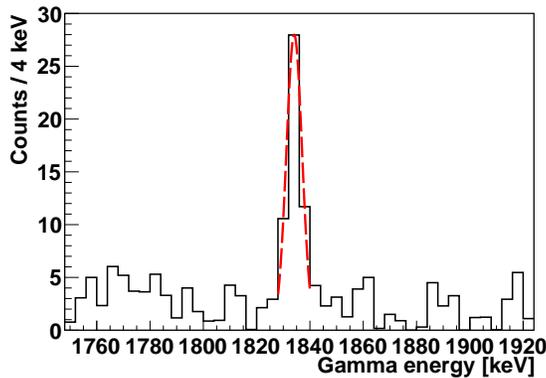
Fig. 3.  $\gamma$ -ray observed at 1835 keV in coincidence with the charged-particle decays correlated with the  $^{56}\text{Zn}$  implants.
