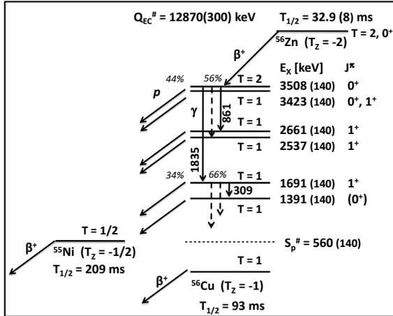
Fig. 4. The  $^{56}\text{Zn}$  decay scheme deduced from the present experiment. Solid lines correspond to observed proton or  $\gamma$  decays. Dashed lines indicate transitions observed in the mirror  $^{56}\text{Co}$  nucleus. The level energies are deduced from our data, having an intrinsic uncertainty of  $\sim 10$  keV. The larger error comes from the uncertainty in the proton separation energy.
