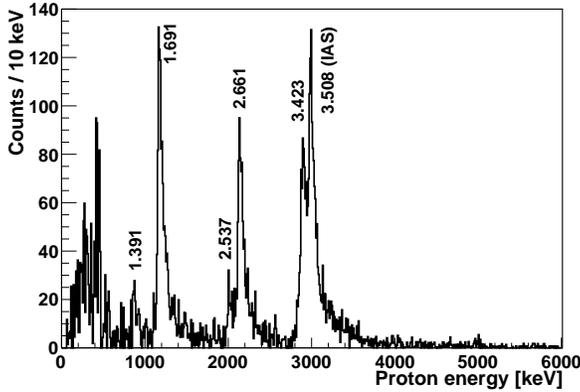
Fig. 1. Charged-particle spectrum measured in the DSSSD for decay events correlated with the  $^{56}\text{Zn}$  implants. The peaks are labeled according to the corresponding excitation energies in  $^{56}\text{Cu}$  (in MeV).
