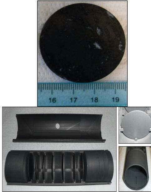
Fig. 3. The SPES multi-foil  $UC_x$  target.
