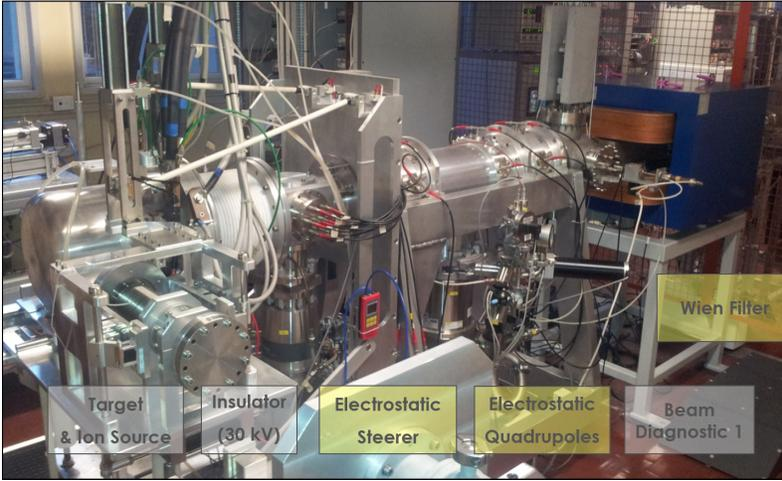
Fig. 4. The SPES test bench: from the left-hand side one can observe the proton beam line, the TIS system, the insulator, the electrostatic steerer, the electrostatic quadrupole and, finally, the Wien Filter selector.
