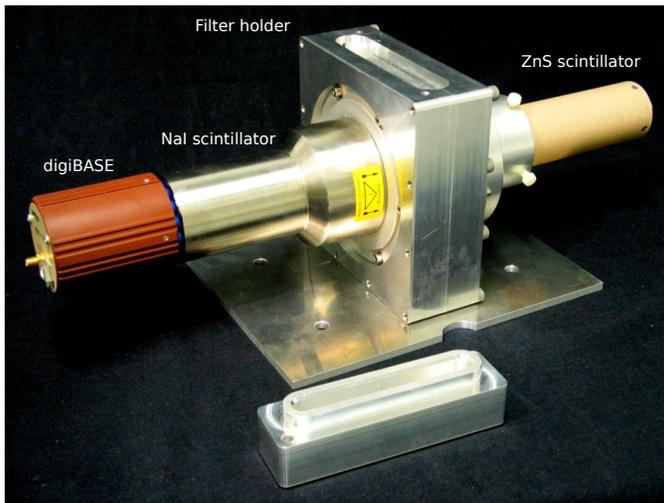
Fig. 2. A setup for the in field detection of  $^{241}\text{Am}$  from air filters [7].
