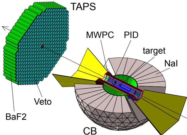
Fig. 1. Experimental setup combining Crystal Barrel (CB, only lower half shown), TAPS, and charged-particle identification detectors. Target in the center of the CB, beam from the lower-right to upper-left corner.
