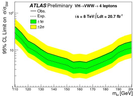
Fig. 3. Upper limits, observed (continuous line) and expected (dashed line), at 95% C.L. on the  $ZH$  production using  $20.7 \text{ fb}^{-1}$  at  $\sqrt{s} = 8$  TeV in the SM Higgs scenario [4]. For the SM Higgs boson at  $m_H = 125$  GeV, the expected and observed limits are respectively 9.6 and 14.3 times the SM cross section.
