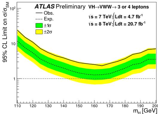
Fig. 4. Upper limits, observed (continuous line) and expected (dashed line), at 95% C.L. on the  $VH$  production using the 3-lepton analysis of the 7 TeV and 8 TeV data and the 4-lepton analysis of the 8 TeV [4]. For the SM Higgs boson at  $m_H = 125$  GeV, the expected and observed limits are respectively 3.6 and 7.2 times the SM cross section.
