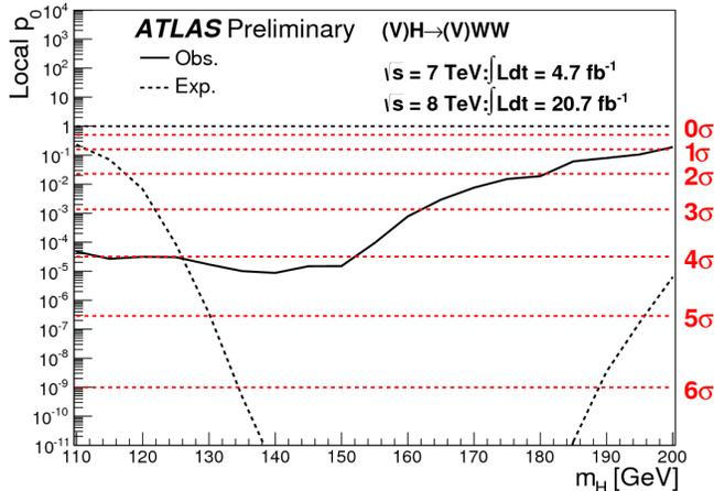
Fig. 5. The observed (continuous line) and expected (dashed line) local  $p_0$  as a function of the hypothesized Higgs boson mass for the combination of  $VH$  and  $H \rightarrow WW^{(*)} \rightarrow l\nu l\nu$  analyses [4].
