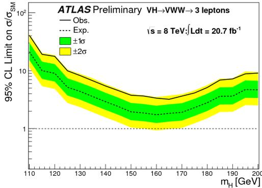
Fig. 1. Upper limits, observed (continuous line) and expected (dashed line), at 95% C.L. on the  $WH$  production using  $20.7 \text{ fb}^{-1}$  at  $\sqrt{s} = 8$  TeV in the SM Higgs scenario [4]. For the SM Higgs boson at  $m_H = 125$  GeV, the expected and observed limits are respectively 5.2 and 10.0 times the SM cross section.
