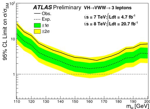
Fig. 2. Upper limits, observed (continuous line) and expected (dashed line), at 95% C.L. on the  $WH$  production using data acquired by the ATLAS experiment up to the 2012 end [4]. For the SM Higgs boson at  $m_H = 125$  GeV, the expected and observed limits are respectively 4.1 and 7.5 times the SM cross section.
