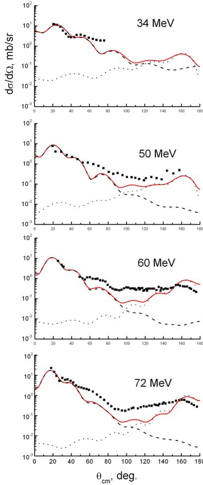
Fig. 4. The angular distributions of the  $^3\text{He}$  ions scattered on  $^6\text{Li}$  nuclei at 34, 50, 60 and 72 MeV energies with excitation of the 2.186 MeV ( $3^+$ ) state. All notations are the same as in Fig. 3.
