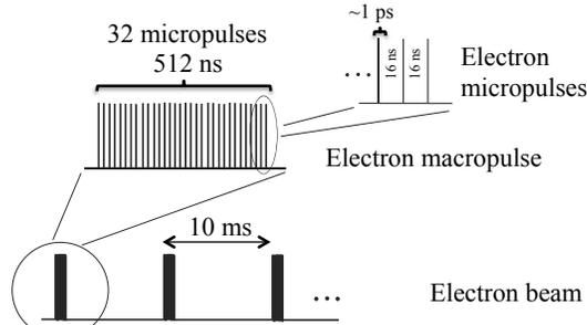
Fig. 3. Time structure of the electron beam provided by the ELI-NP normal conducting linac. The RF repetition rate is of 100 Hz. At every RF pulse, a train of 32 electron micro-bunches, with 250 pC charge and about 1 ps time duration each, is generated. The time separation between the micro-bunches is of 16 ns.
