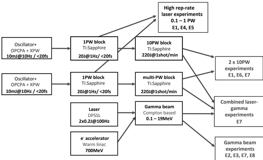
Fig. 4. Block diagram of the ELI-NP facility.
