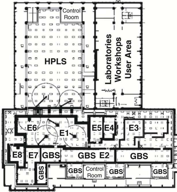
Fig. 1. A schematic layout of the ELI-NP experimental building showing the main areas for the implementation of the research equipment and support laboratories. The meaning of the labels is as follows: HPLS — high-power laser system, GBS — gamma beam system, E1...E8 — experimental rooms.
