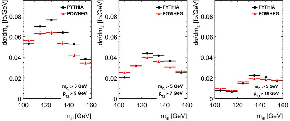
Fig. 5. The  $4\mu$  channel PYTHIA and POWHEG differential cross sections as a function of  $m_{4l}$  for  $m_{Z_2} > 5$  GeV and the minimal  $p_{T,l}$  cut values: (left) 5 GeV, (middle) 7 GeV, and (right) 10 GeV. The PYTHIA cross sections are corrected for the missing interference effects using the ratios of the POWHEG distributions obtained by including and excluding the interference effects in the event generation.
