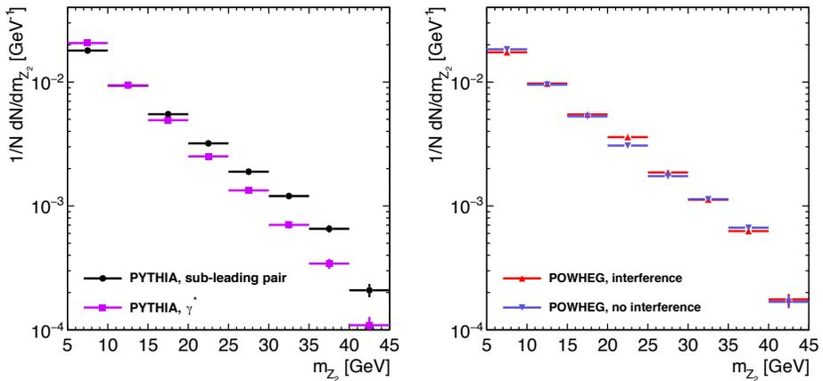
Fig. 4. (Left) The comparison of the PYTHIA distributions of the invariant mass  $m_{Z_2}$ : (1) for the  $Z_2$  pairs found algorithmically, and (2) for  $Z_2$  the pairs coming from conversions of virtual photon emitted by leptons and quarks. (Right) The comparison of the POWHEG distributions of the invariant mass  $m_{Z_2}$ : (1) including and (2) excluding the interference effects.
