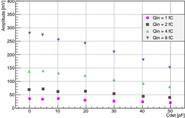
Fig. 7. SALT response as a function of a detector capacitance for a given time of 26 ns.
