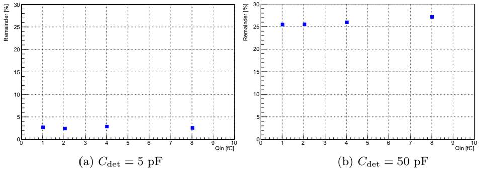
Fig. 6. Remainders as a function of injected charge for the detector capacitances ( $C_{det}$ ).
