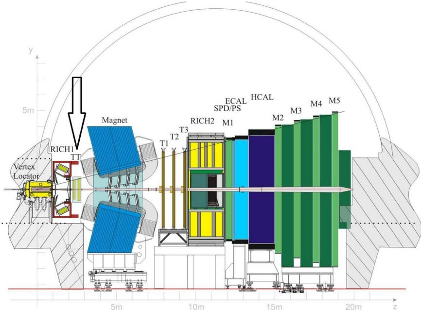
Fig. 1. Layout of the LHCb spectrometer. The arrow indicates the TT detector [1].
