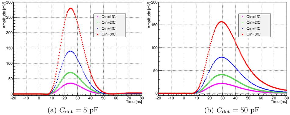
Fig. 5. SALT response as a function of time for the given detector capacitances ( $C_{det}$ ) for variety of injected charges ( $Q_{in}$ ).
