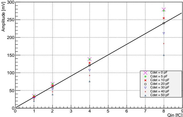
Fig. 8. SALT response as a function of an injected charge for a given time of 26 ns.
