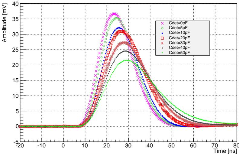
Fig. 4. SALT response as a function of time for the injected charge  $Q_{in} = 1$  fC for variety of capacitences.
