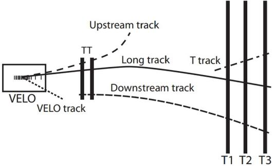
Fig. 2. Track definitions as used by the LHCb Experiment [2].
