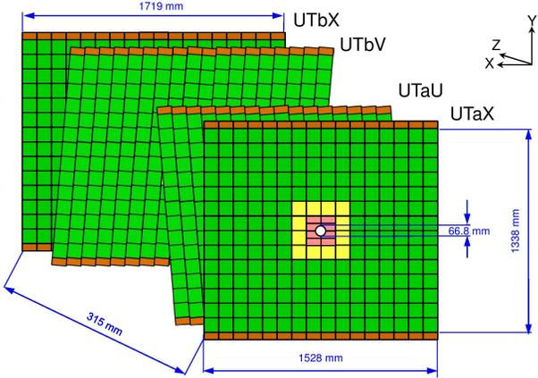
Fig. 3. Scheme of four sensor layers in the UT detector [5].
