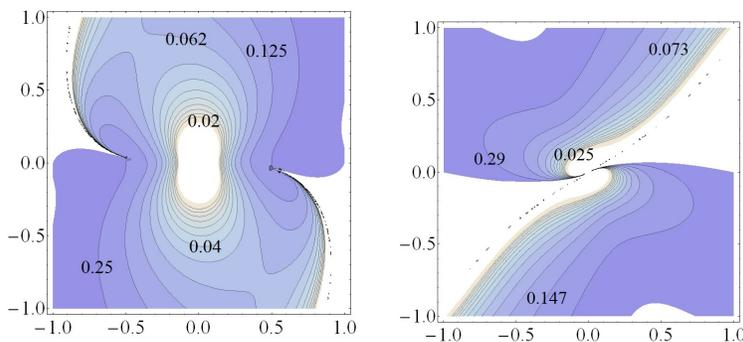
Fig. 4. Sectional view of the force-free surface for  $\alpha = \frac{\pi}{6}$  in the plane  $\psi = \frac{\pi}{2}, \frac{3\pi}{2}$  (left), and in the plane  $\psi = 0, \pi$  (right) for different values of the radius of the sphere  $a$ . The values of  $a$  are marked in the figures.
