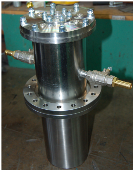
Fig. 9. Photograph of a part of beam-forming system designed and manufactured at the NCBJ. Aluminum flattening foil is visible in the center, on the top of the steel flange on entry to the applicator tube. A flange visible in the middle of the applicator is for connecting the applicator with the LN 2 cryostat, as discussed in Sec. 3.
