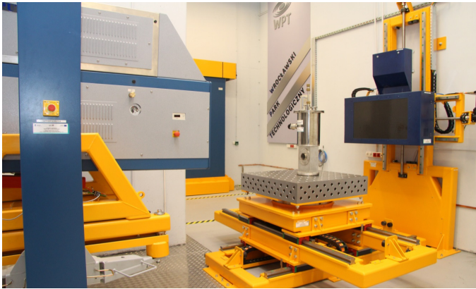
Fig. 1. The LILLYPUT 3 system in a standard radiographic configuration installed at the Nondestructive Testing Laboratory at Wrocław Technology Park. The accelerator is visible on the left-hand side, the object table in the center and digital imaging system on the right-hand side.
