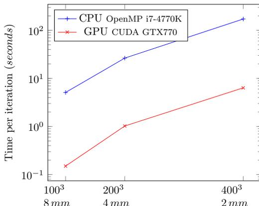
Fig. 2. CPU vs. GPU implementation — single image reconstruction iteration time as a function of target image resolution.
