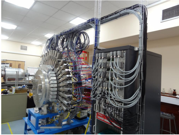
Fig. 2. LYCCA chamber with the large stop detector and the FEE cards wired and mounted on the horseshoe structure at Daresbury.
