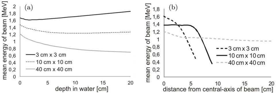
Fig. 3. The mean energy of the 6 MV X-ray beam from the Clinac 2300 (a) *versus* the depth along the beam central-axis in water and (b) *versus* the distance from the central-axis of the beam at the depth of 1.5 cm, for various radiation fields and SSD = 100 cm.
