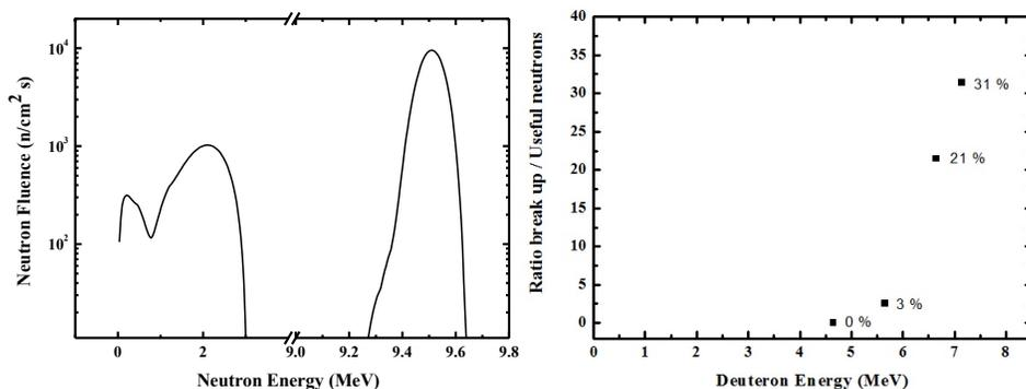
Fig. 4. (Left) The calculated neutron energy spectrum for 9.5 MeV. (Right) The ratio of parasitic neutrons produced from the breakup reaction to the neutrons produced from the  $^2\text{H}(d, n)$  reaction.
