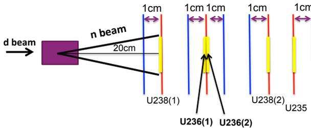
Fig. 1. (Color online) Schematic views of the gas cell, the target (light gray/yellow) and detector (dark gray/blue) assembly.
