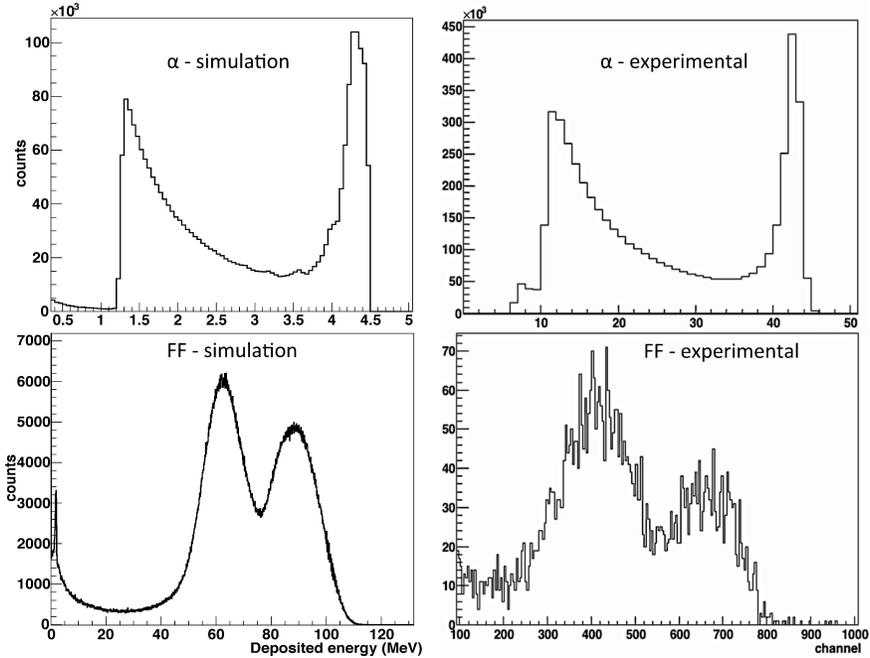
Fig. 3. Comparison of the simulated energy deposition histograms with the corresponding experimental spectra for  $\alpha$  particles (upper figures) and FFs (lower figures).
