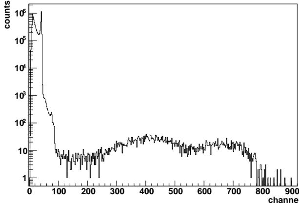
Fig. 2. A typical spectrum obtained for one of the  $^{236}\text{U}$  targets at  $E_n = 10$  MeV.
