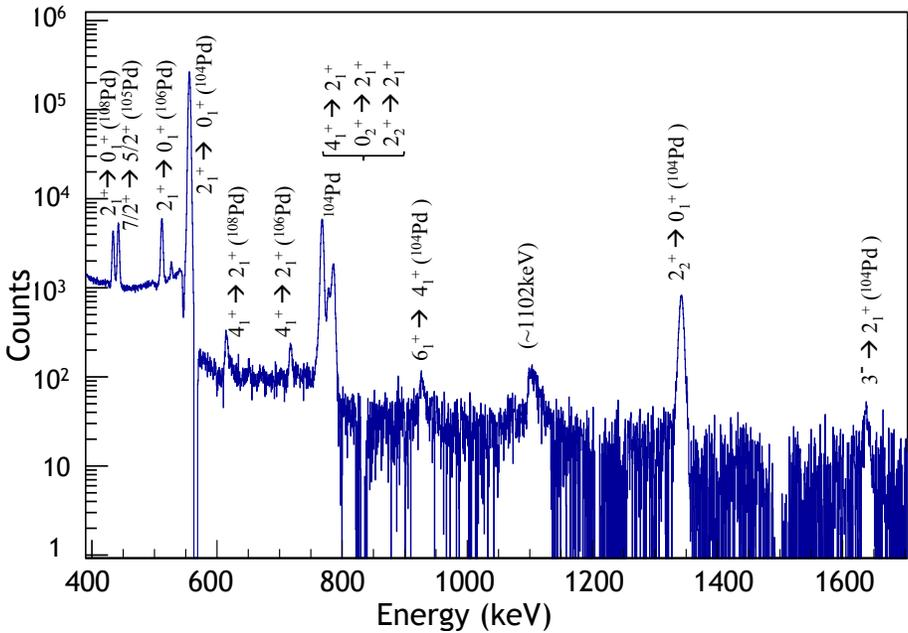
Fig. 3. Total background-subtracted and Doppler corrected gamma-ray spectrum resulting from present Coulomb excitation experiment of  $^{104}\text{Pd}$  with 91 MeV  $^{32}\text{S}$  beam. The 1102 keV peak was not interpreted within the known level schemes of palladium isotopes; its interpretation will be subject of the further analysis.
