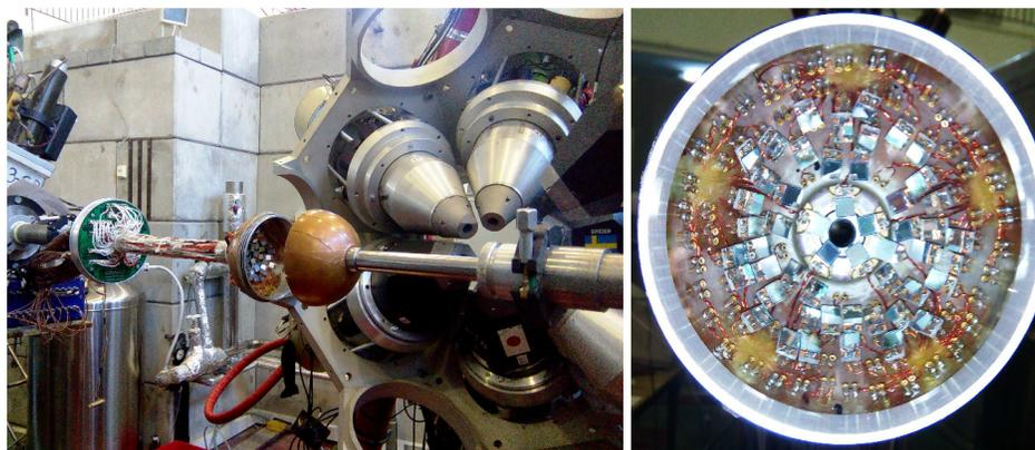
Fig. 1. Open view of the PIN-diode array mounted at the centre of the EAGLE spectrometer [13] (left). PIN-diodes of  $0.5 \times 0.5\text{ cm}^2$  active area mounted inside the scattering chamber [14] (right).
