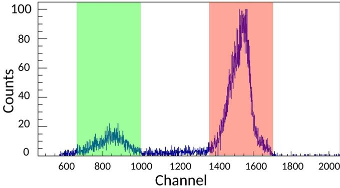
Fig. 2. Particle- $\gamma$  coincidence timing spectrum for individual PIN-diode-HPGe combination for the pulsed beam from the Warsaw cyclotron. Gates on the random and prompt peaks are shown by the shaded regions from channel numbers 650–1000 and 1350–1700, respectively. The spectrum is calibrated with 0.1 ns per channel.
