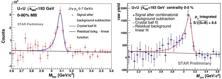
Fig. 2.  $J/\psi$  signal after combinatorial background subtraction fitted with a crystal ball function together with a linear function used to describe the residual background in minimum bias (left) and 0–5% central (right) U+U collisions.
