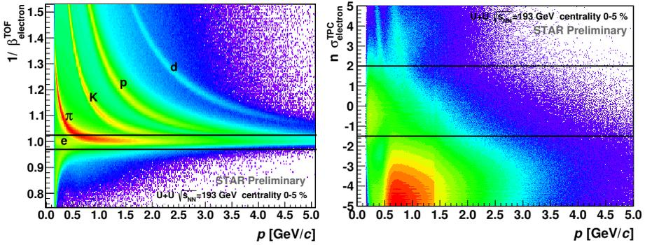
Fig. 1. Left:  $1/\beta^{\text{TOF}}$  of particles with depicted cut for electron candidates (black lines). Right:  $n\sigma_e^{\text{TPC}}$  of particles satisfying TOF and BEMC cuts, black lines denote the  $n\sigma_e^{\text{TPC}}$  cut.
