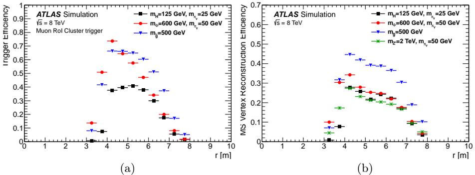
Fig. 3. Barrel efficiency as a function of the radial decay position of the long-lived particle for (a) the Muon RoI Cluster trigger and (b) MS vertex reconstruction for scalar boson, for a selection of simulated benchmark signal samples [2].
