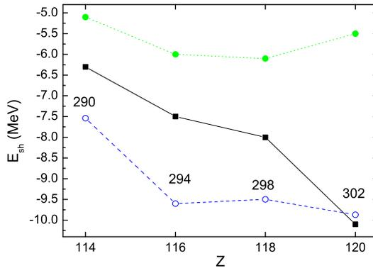
Fig. 8. Shell corrections to the binding energies of the nuclei of  $\alpha$ -decay chain of  $^{302}120$ . The results of the TCSM [14] are shown by solid squares connected by solid line. The results of Ref. [8] are presented by solid circles. The values of  $E_{\text{sh}}$  obtained for the Woods–Saxon potential extracted from the self-consistent microscopical calculations are shown by open circles.
