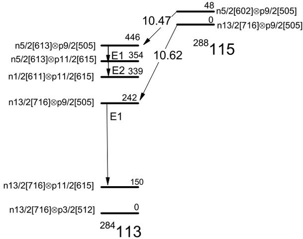
Fig. 5. Decay scheme of  $^{288}\text{Mc} \rightarrow ^{284}\text{Nh}$  resulting from the calculations with the TCSM model. Energies of two-quasiparticle levels are in keV,  $Q_\alpha$  values are in MeV. The most probable gamma transitions are marked.
