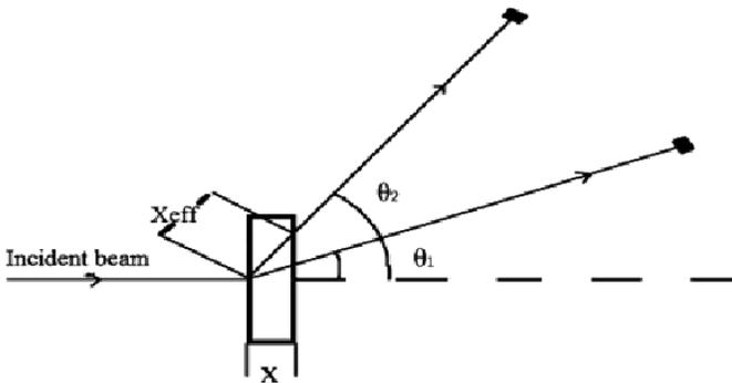
Fig. 1. Geometry for measuring the scattering process by a thin foil.
