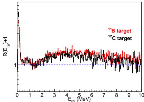
Fig. 4.  $\alpha$ - $\alpha$  correlation function obtained with the FARCOS device from  $^{16}\text{O}$  (55 MeV/ $u$ ) on  $^{12}\text{C}$  and  $^{11}\text{B}$  targets data.
