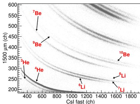
Fig. 3. A  $\Delta E-E$  (DSSSD,  $1500\ \mu\text{m}$ -CsI) identification matrix obtained with FARCOS. Arrows and labels indicate lines corresponding to the firsts lightest isotopes identified.
