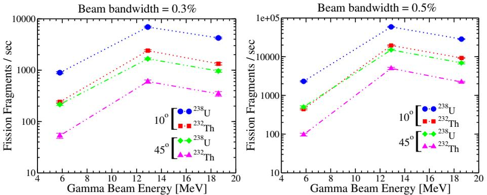
Fig. 1. Estimated fission fragment emission rates for the ELI-NP gamma beam on  $^{238}\text{U}$  and  $^{232}\text{Th}$  targets of thickness of  $20\text{ mg/cm}^2$ , for three  $\gamma$ -beam energies, 5.8, 12.9, and 18.6 MeV. Results for a beam bandwidth of 0.3% (left) and 0.5% (right) are shown. The statistical uncertainties are smaller than the symbols.
