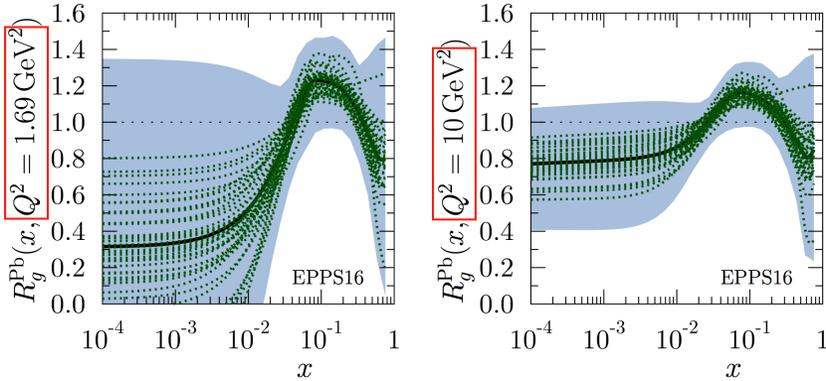
Fig. 1. The EPPS16 nuclear modifications for lead. Largest uncertainty for gluon distributions is for  $x < 10^{-2}$  and low  $Q^2$ . This is because of a lack of data in this region. Dotted lines show different contributions to the uncertainties [1].
