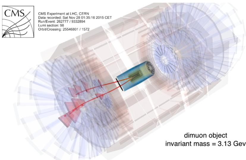
Fig. 6. The event display shows one of the selected events, the visualisation of the CMS detector can be seen, together with two trajectories of muons going into forward direction. The reconstructed invariant mass of the two leptons is about the  $J/\psi$  mass.
