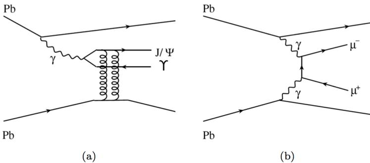
Fig. 2. The Feynman diagrams of an UPC for PbPb. Diagram (a) shows photoproduction process of vector mesons, (b) is a  $\gamma\gamma$  interaction producing two muons, the main background to the analysed process.
