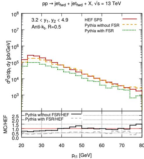
Fig. 3. Transverse momentum distribution in forward-dijet production — comparison between HEF (DLC2016) and PYTHIA.
