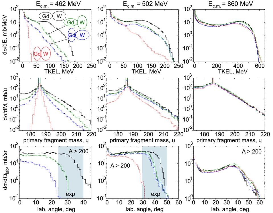
Fig. 1. Total kinetic energy loss, mass, and angular distributions of primary products of the  $^{160}\text{Gd} + ^{186}\text{W}$  reaction calculated at three energies  $E_{c.m.} = 462, 502,$  and  $860$  MeV. Solid, dashed, dash-dotted, and dotted histograms correspond to tip-to-tip, tip-to-side, side-to-tip, and side-to-side collisions. Shaded areas in the angular distributions show the angular ranges covered in the experiment [11].
