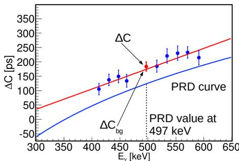
Fig. 4.  $\Delta C$  values for the background at different energies around the peak at 497 keV (lighter/blue dots). The straight/red line is the linear fit of these values, obtained via a weighted  $\chi^2$  minimization algorithm. The darker/red dot represents the  $\Delta C$  value for the  $6^+ \rightarrow 4^+ \rightarrow 2^+$  cascade.  $\Delta C_{\text{Bg}}$  was calculated to be 174 ps at the energy of 497 keV. The PRD curve is represented by the solid/blue line.
