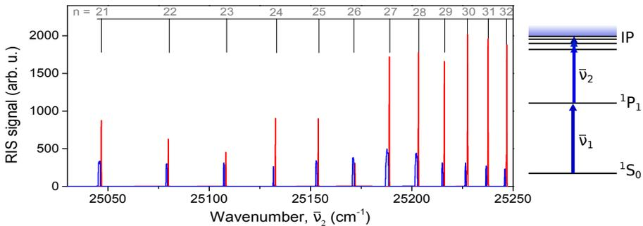
Fig. 1. Left panel: The measured Rydberg states in Yb at 5 mbar (lighter/red line) and 200 mbar (darker/blue line) plotted against the wavenumber ( $\bar{\nu}_2$ ) along with their respective principal quantum number ( $n$ ) on top. Right panel: Simplified ionization scheme.
