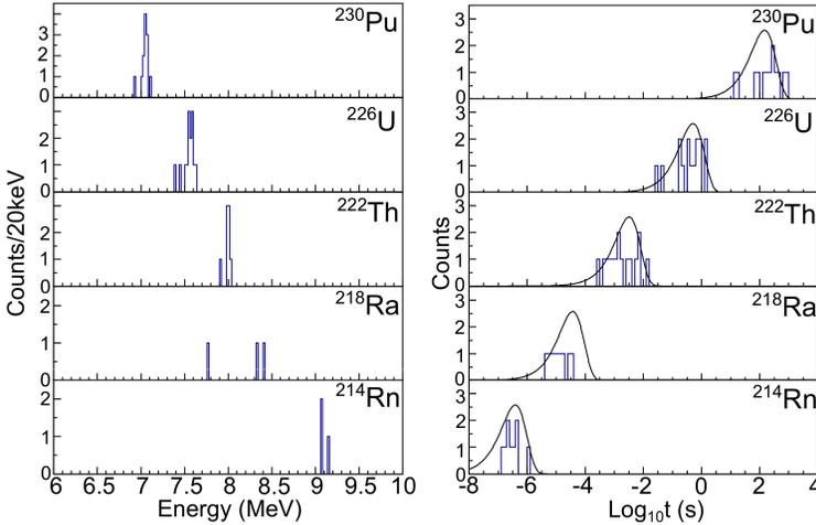
Fig. 4. Left: The  $\alpha$ -decay energies of the decay chain originating from  $^{230}\text{Pu}$  measured at SHIP. Right:  $\alpha$ -decay half-life distributions of each member of the chain. The solid curves indicate the calculated time distributions for which the mean values are taken from literature.
