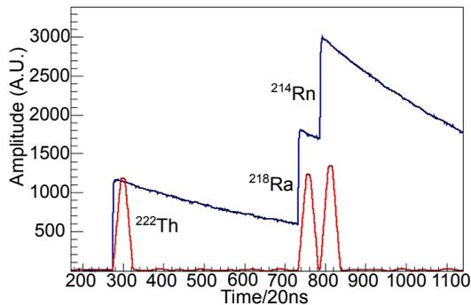
Fig. 2. (Colour on-line) An example trace (black/blue) of the triple pile-up signal  $^{222}\text{Th}$  ( $1.56 \text{ ms}$ )  $\rightarrow$   $^{218}\text{Ra}$  ( $9.17 \mu\text{s}$ )  $\rightarrow$   $^{214}\text{Rn}$  ( $1.09 \mu\text{s}$ ) with the energy resolved using the trapezoidal filter shown in grey/red, and the times given as the measured values in the shown trace.
