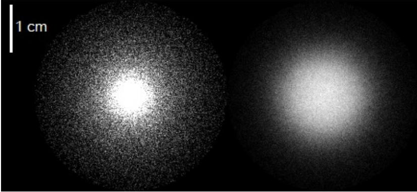
Fig. 3. Spatial projections of dose distribution in water from point-like sources of  $^{11}\text{C}$  (left) and  $^{34m}\text{Cl}$  (right).
