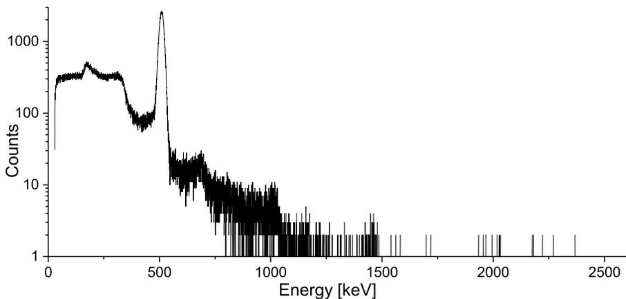
Fig. 2. Gamma-ray energy spectrum of liver irradiated with a dose of 500 Gy measured with a LaBr<sub>3</sub> detector. The measurement started 10 minutes after irradiation and lasted for 100 seconds.
