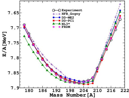
Fig. 8. Binding energies of even-even Pb isotopes calculated in the RHB model with the mean-field effective interactions DD-ME2, DD-PC1, and NL3\*, and with the separable pairing model. The theoretical binding energies are compared with the experimental data [97, 98], FRDM [99], and HFB [100].
