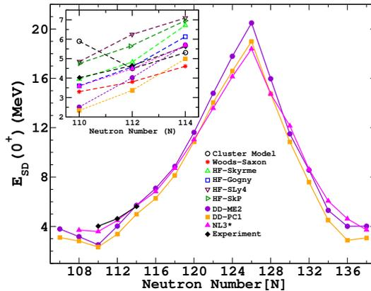
Fig. 12. Experimental and theoretical SD bandhead energies. Present results with the DD-ME2, DD-PC1, and NL3\* effective interactions, and with the separable pairing, are compared with other model predictions and the experimental data [71] (insight of the figure). Strutinsky method using a Woods–Saxon potential [73]; HF-Skyrme, HF-SLy4, HF-SkP, and HF-Gogny: HFB using density-dependent Skyrme [74], SLy4 [76], SkP [76], and Gogny [77] interactions; cluster model [78].
